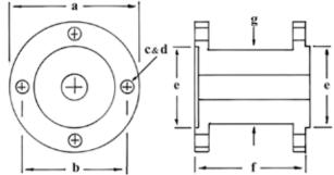
R&D Marine can provide a Bobbin to extend the shaft. If the gearbox fitting you require is not listed please contact PYI Inc.
