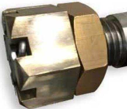
For decades there has been a nut available that is specifically designed to be held in place with a cotter pin. It is called a castle nut or castellated nut. In most cases these nuts have to be custom made in a machine shop for each propeller and shaft setup for everything to line up correctly due to the limited depth of the notches.
