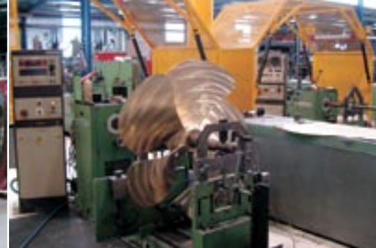
A VEEMStar ® propeller being balanced in one of VEEM's 7 balancing machines
