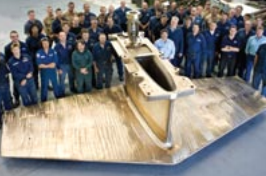
Hollow section ride control "T" foil as fitted to Austal Ships vessel
