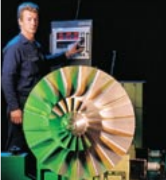
Precision dynamic balancing of rotor components
