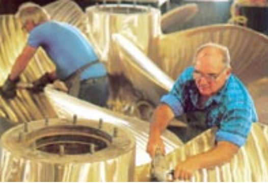
The sea of gold – propeller finishing. Destroyer escort propellers manufactured from nickel aluminium bronze. The end result is spectacular!
