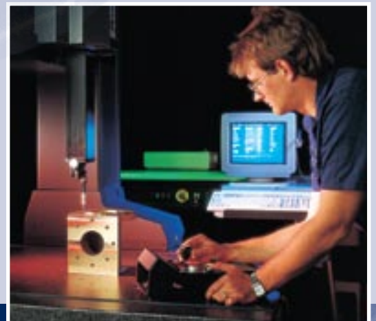
Dimensional inspections of all types of components can be carried out using a computerised coordinate measuring machine
