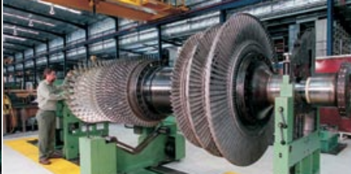
VEEM has NATA certification for dynamic balancing up to 28 tonne – refurbished GE gas turbine rotor
