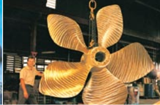
Royal Australian Navy Destroyer Escort propellers repaired at VEEM
