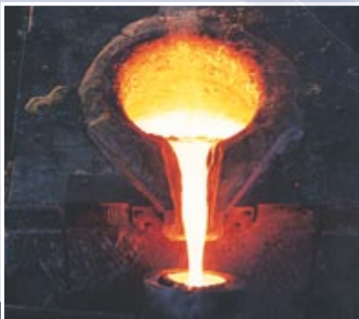
14 tonne melting capacity of bronzes
